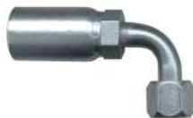
90° ELBOW S.A.E. 37° Female Flare (Swivel)
