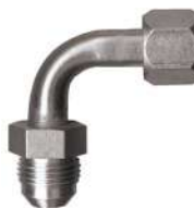
90° BENT TUBE ELBOW Female 37° Swivel To Male JIC
